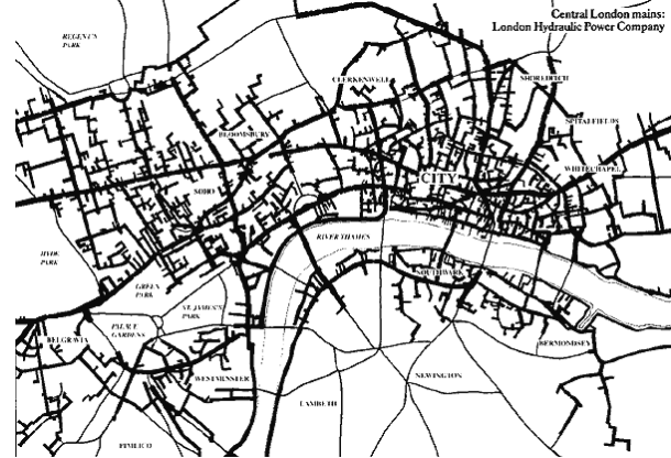
Figure 25: London Hydraulic Power Company network
