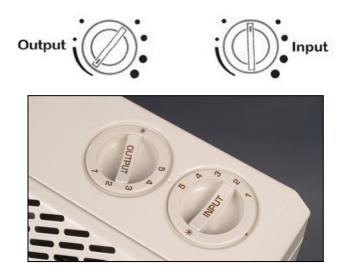
The **Input control dial**, which should be on the *right hand side*, controls how much the heaters charge-up overnight and during the afternoon, with `5/6' being the highest setting.
